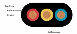
These submersible flat cable are specially designed to provide distinguished tube like structure for the insulated cores. The wall between the cores perfectly separates them from coming in contact with each other and provides better mechanical and electrical strength compared to the traditional submersible flat cables. The knurling on the outer surface makes the cable more durable and provides improved abrasion resistance during handling and installation of these cables.
